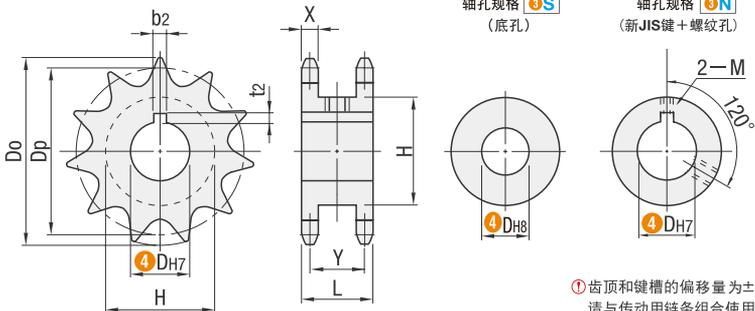
①齿顶和键槽的偏移量为±0.5mm
